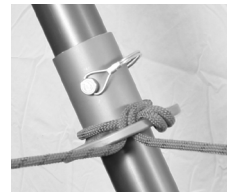
Fig 24 Lash Ring used near foot section for increased stability
