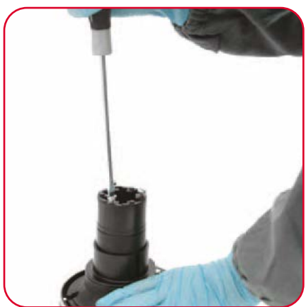
7. Completely unscrew three screws
