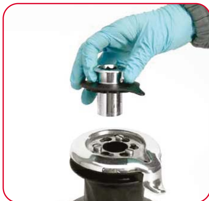
2. Slide off the hub n°20 and the cover n°19
