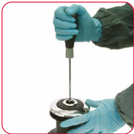
1. Unscrew the central screw (2Nm/18in-lb)
