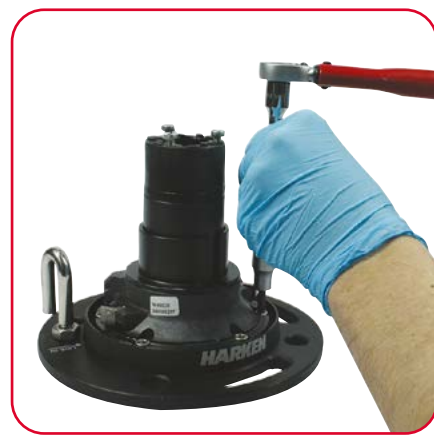
6. Unscrew the five screw (8Nm/71in-lb) and remove the plate
