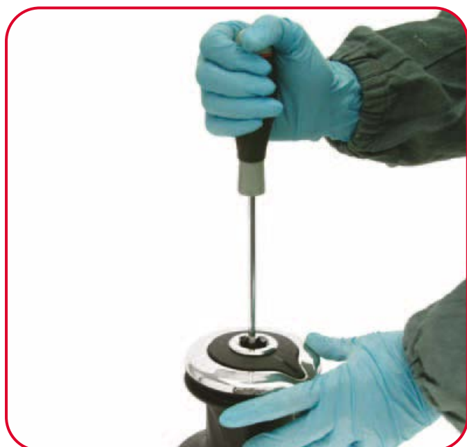
1. Unscrew the central screw ( 2 Nm/18 in-lb)
