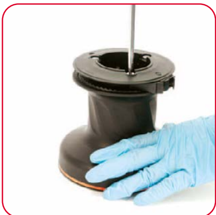
1. Unscrew the 3 screws (4 Nm/35 in-lb)
