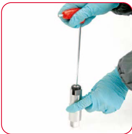
13. Unscrew the screw and remove the washer (4 Nm/35 in-lb)
