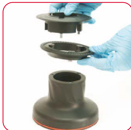
2. Remove the jaws from drum
