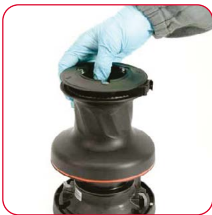
5. Lift off the drum
