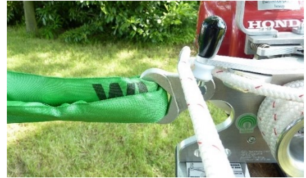
Fig.5: Guiding the rope through the clamp
