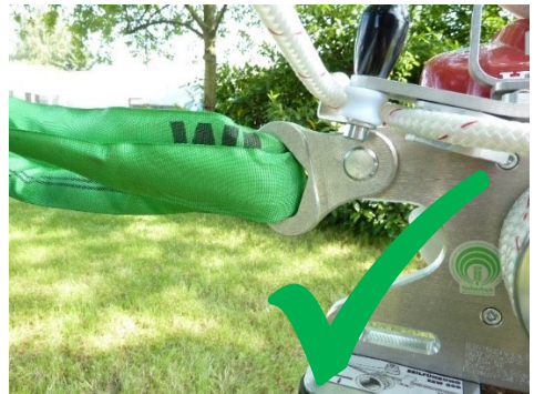
Fig.7: Correct fastening the EDER Powerwinch 500
