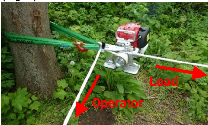
Fig.4: EDER Powerwinch 500 in working position
