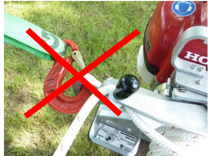
Fig.6: wrong fastening the EDER Powerwinch 500
