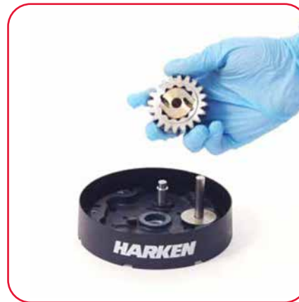
17. Remove the pawls. To facilitate the operation press the spring against the pawl with a blade.
