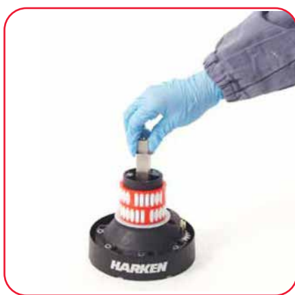
9. Slide out the central shaft
