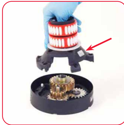
11. Remove the drum support. Note down serial number of winch and record.
