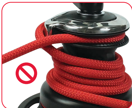
Excessive turns at base of winch
