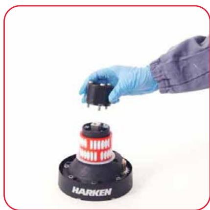
8. Remove the self-tailing arm support and slide out the bushing
