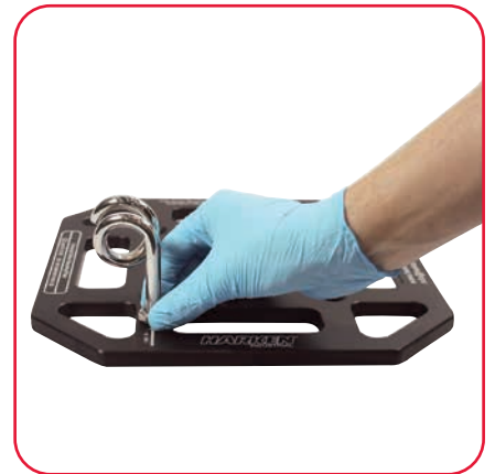
3. Wind nut back down onto plate to lock pigtail in place with the end of the pigtail spiralling towards the winch line entry point
