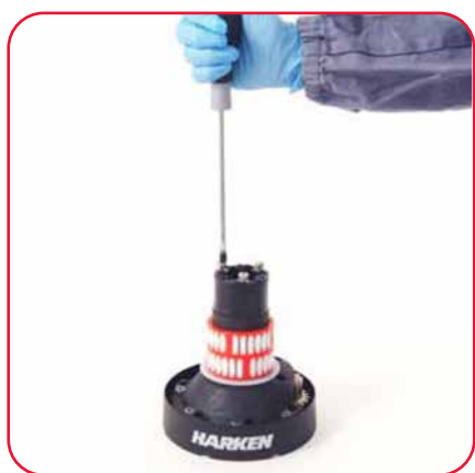
7. Completely unscrew three screws
