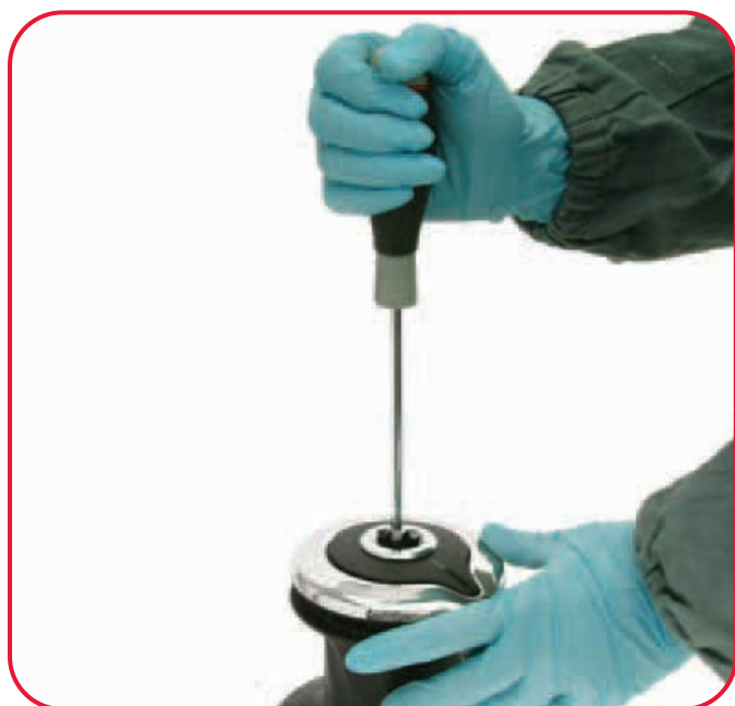
1. Unscrew the central screw ( 2 Nm/18 in-lb)
