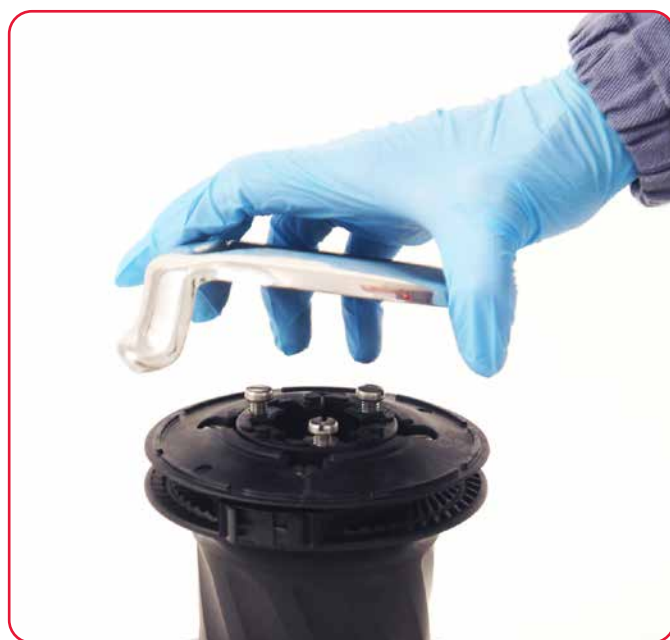
4. Remove the self-tailing arm by rotating and lifting it.
