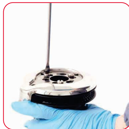
3. Unscrew the three screws (4Nm/35in-lb)
