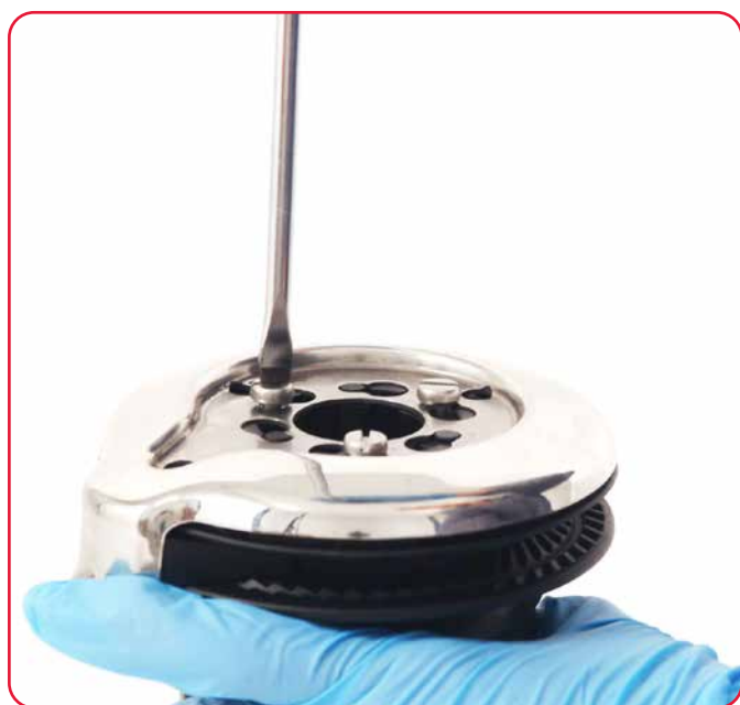
3. Unscrew the three screws (4Nm/35 in-lb).
