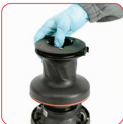
5. Lift off the drum
